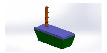
Impermeable cover preventing the emission of dust generated by the exit of the rubble and the deposit in the dumpster of waste foreign to the site.
